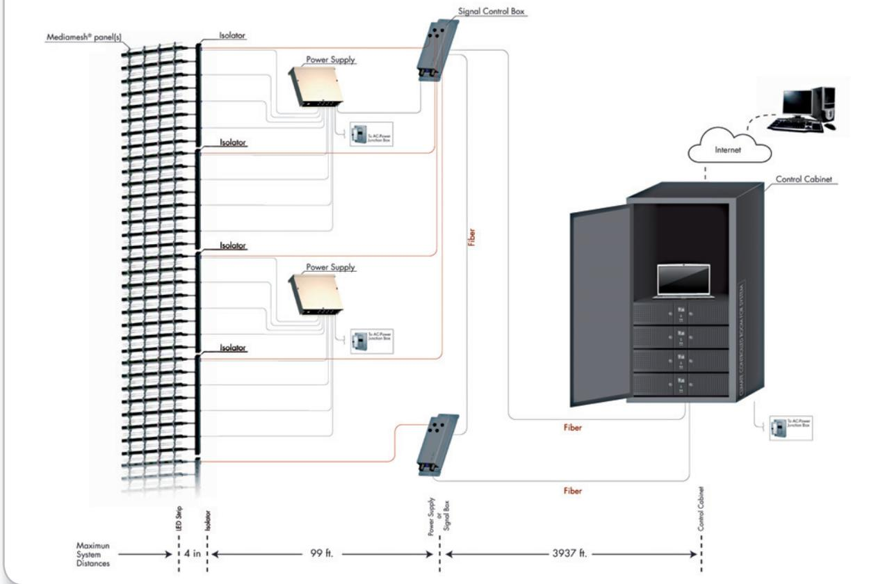
Cabling of the 6 LEDs per pixel system rows and supply of power and programming data
