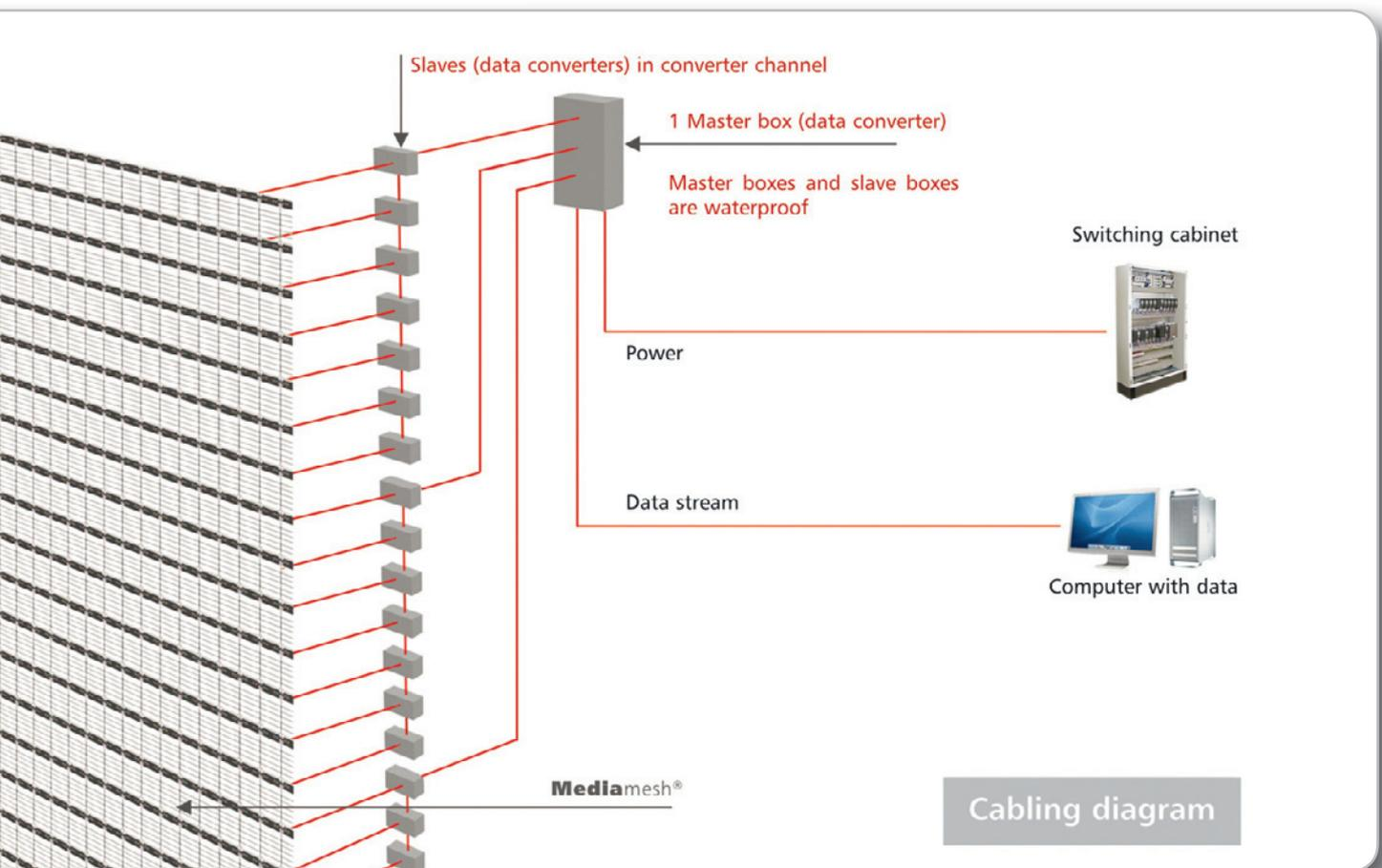
Cabling of the 5 LEDs per pixel system rows and supply of power and programming data
